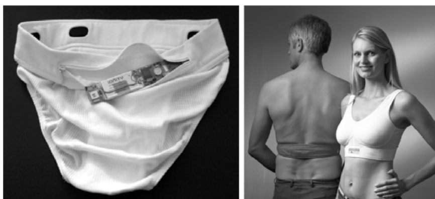
Figure 6.1-13. Flexible ECG monitoring device appropriate for integration into underwear (left), textile belts or bras (right). (Copyright Philips Research Aachen, modified and reprinted by permission.)
