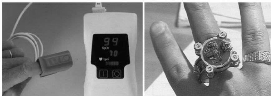
Figure 6.1-15. Classical handheld pulse oximeter (left, [19]) (Copyright Nellcor Puritan Bennet Inc. USA and the miniaturized Harvard saturation measurement ring right, from [18]. Modified and reprinted by permission.)
