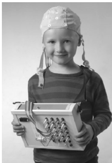
Figure 2.3–3. Child carrying the first-generation ambulatory EEG transmitter.
