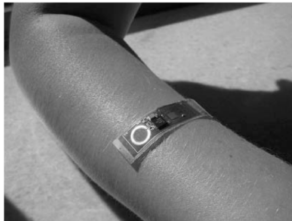
Figure 2.3–10. Prototype sensor in a flexible band aid.
