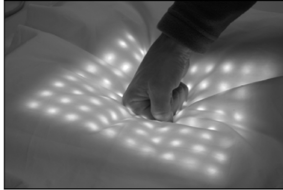
Figure 1.2-4. Textile photonics: LED's integrated into a pillow.
