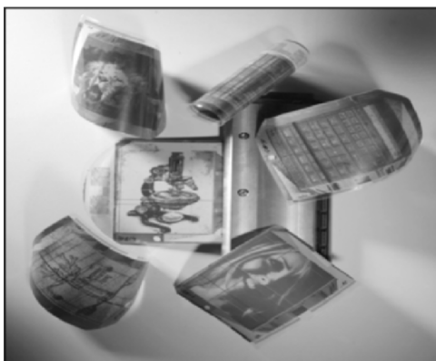
Figure 1.2-1. A rollable display using a polymer electronics active matrix.
