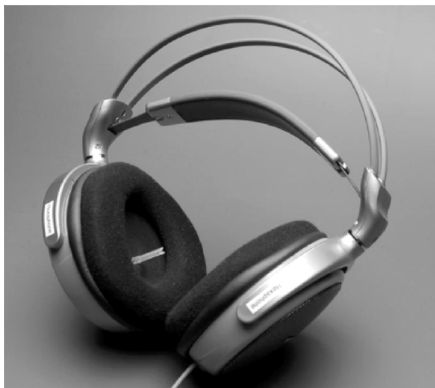
Figure 6.3-8. Prototype of headphones with integrated microphones.
