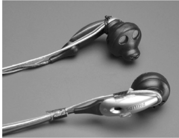
Figure 6.3-9. Prototype of earphones with integrated microphones.
