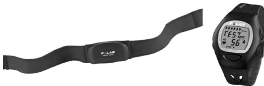
Figure 6.1-9. POLAR thoracic belt (left) and wrist-worn display (right). (Modified from [14], reprinted by permission.)
